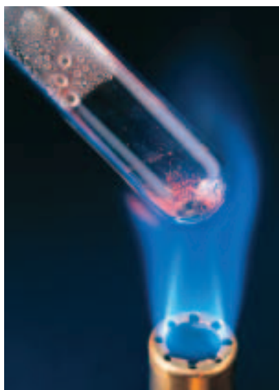
Figure 7 Mercury metal forms when mercury oxide is heated. Because mercury is poisonous, this reaction is never performed in a classroom laboratory.
