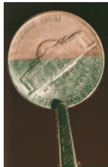
Figure 19 Electroplating of a metal is an endergonic reaction that requires electricity. A coating of copper was plated onto this coin.
