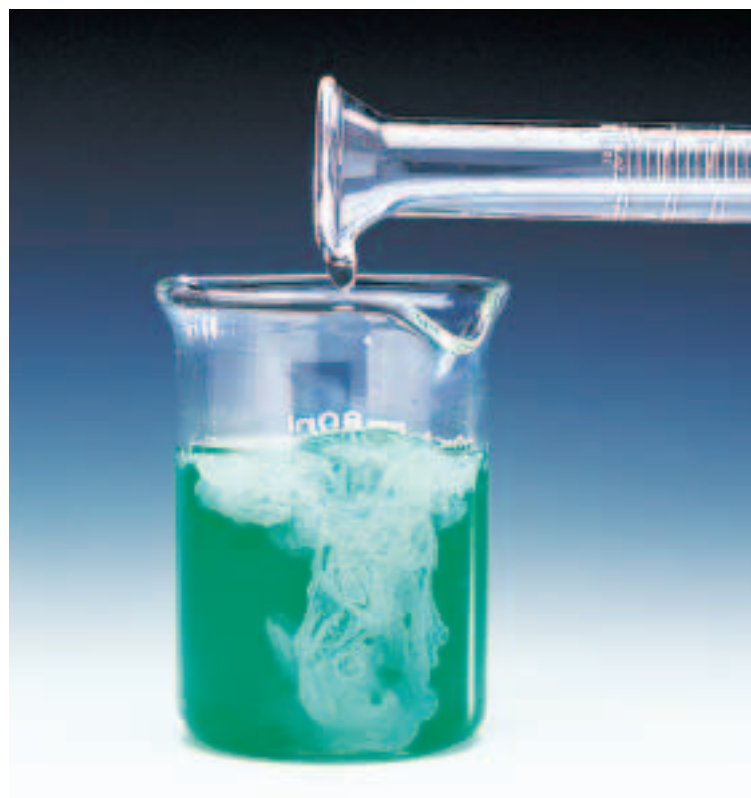
Figure 4 A white precipitate of nickel(II) hydroxide forms when sodium hydroxide is added to a green solution of nickel(II) chloride. Sodium chloride, the other product formed, is in solution.
